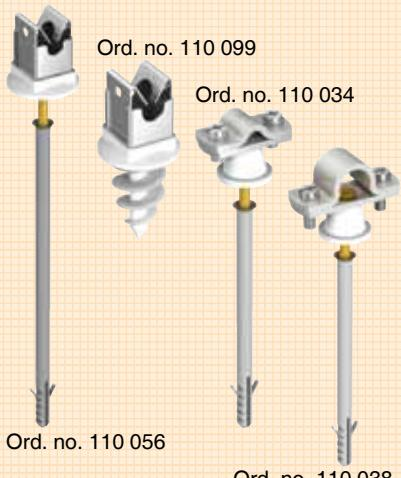
Conductor fastener for round conductor ø 8-10 mm, mounted with screw M6 V2A, washer or spacer, fastening screw and ø 8 mm dowel.
