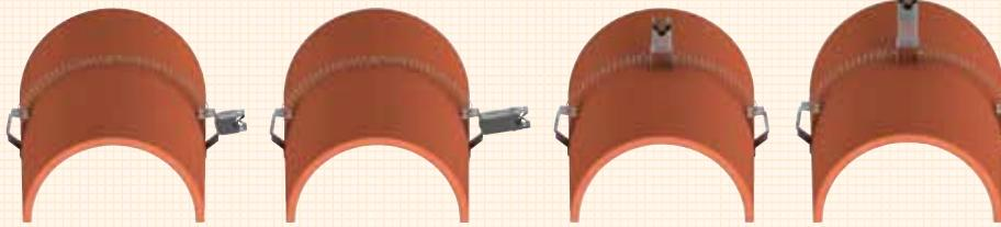
\*) **Type A (I)** = fixed conductor leading; **Type B (II)** = loose conductor leading
