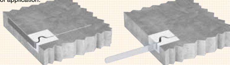
Expansion strip, for a connection of the foundation earth electrode outside the concrete.
