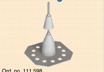
**Roof conductor holder** for synthetic roofing membranes and bitumen roofs. To be fixed onto synthetic roofing membranes with weldable fastening strips; glued directly onto bitumen roofs (PA 6 = Polyamid 6).
