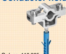
**Rod holder** for fixing air termination rods and earth lead-in rods, with screws M6 V2A, washer or spacer, fixing screw and ø 8 mm dowel.
