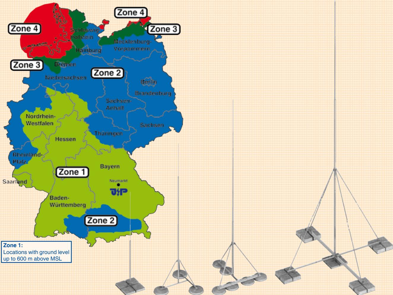
The right base frame for your air termination pole and the appropriate concrete base
